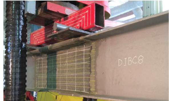
Repaired section prepared for testing
