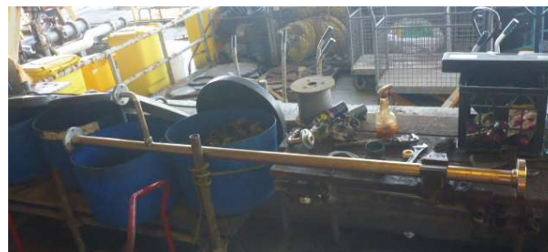
Replacement spools made up on the deck – as required
